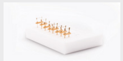
Figure 2: An inside view of HF-QCM and TF Sensor Matrix
